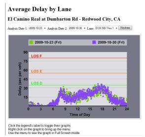
The signal timing and traffic volume information was transmitted to the TrafInfo server at the end of each signal cycle. The central server software logs the information into a MySQL® database, and computes the control delay as per procedures within the Highway Capacity Manual.
